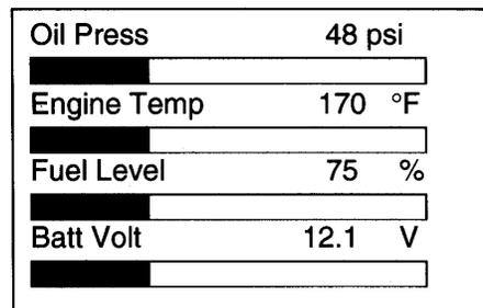
This screen displays the engine operational data of the generator set.
