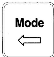
Use this button to scroll the generator operation mode from AUT-MAN-OFF.
