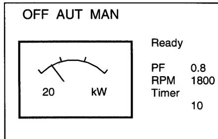
This is the primary optional screen which identifies the status of the generator set along with the generator kW, power factor, and engine RPM.
