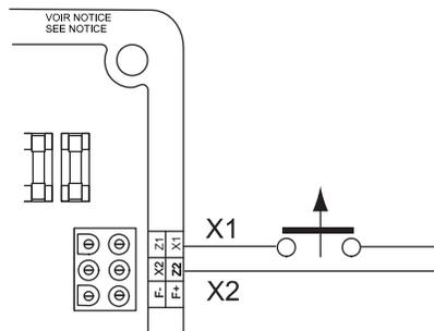
The exciter is switched off by disconnecting the AVR power supply (1 wire-X1 or X2). Contact rating 16A-250V A.C.
