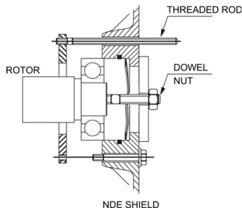
**Replacing the NDE bearing on a single-bearing machine**
