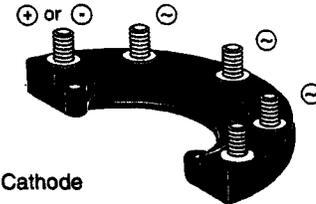
A diode in good condition enables the current to flow in only one direction from Anode to Cathode
