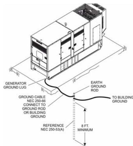
If used as an alternate power supply, connect only after the main service entrance switch has been DISCONNECTED and LOCKED OPEN. In addition, circuit overload protection must be provided in accordance with National Electrical Codes and local regulations.
