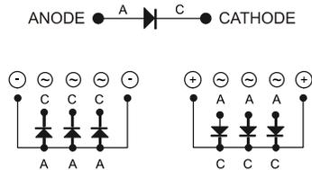
**Checking the windings and rotating diodes using separate excitation**
