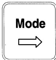
Use this button to scroll the generator operation mode from OFF-MAN-AUT.
