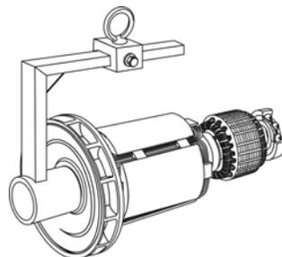
Follow the procedure for reassembling the bearings.
