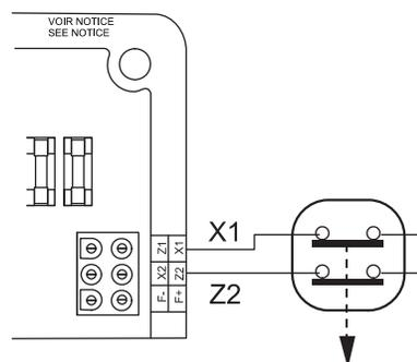
The exciter is switched off by disconnecting the AVR power supply (1 wire on each auxiliary winding). Contact rating 16 A-250V A.C. Connection is identical for resetting the AVR internal protection.
