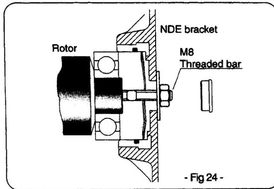
**Replacing the NDE bearing on a single-bearing machine**
