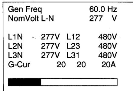
This screen displays electrical values of the generator set. These values include frequency, line voltages, phase voltages, and current per phase.
