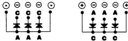
A diode in good working condition allows the current to flow in only one direction, from anode to cathode.
